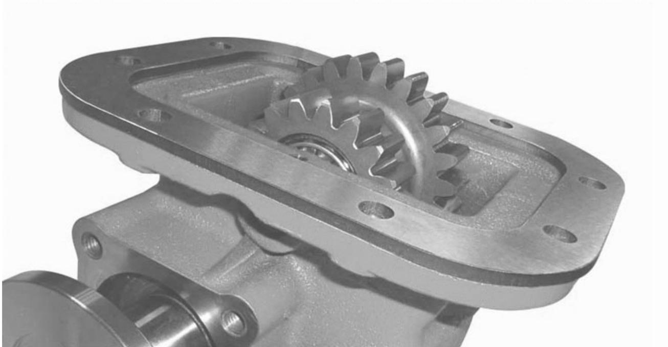
*Figure 2 - PTO example for Endurant XD Series Transmission*
