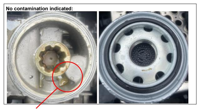
Note: Moisture (Water) droplets found on the cartridge base is normal.
