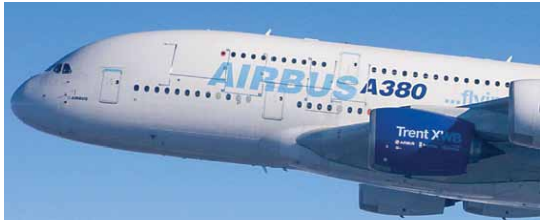
Trent XWB engine on an A380 test aircraft, with expected entry into service in 2014.
