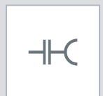
Capacitive voltage detection system
