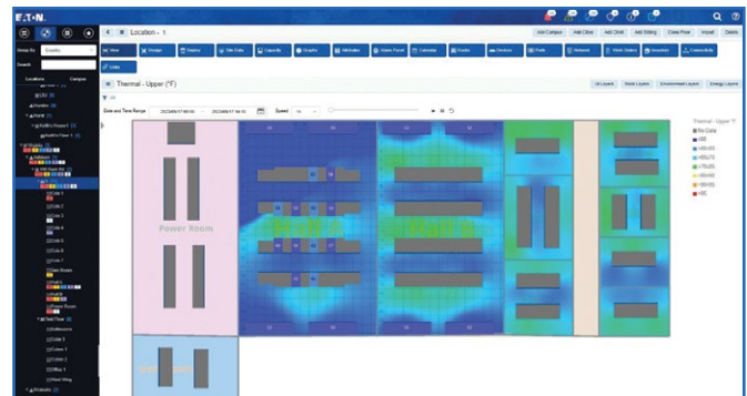
Data center thermal map from DCPM software.
