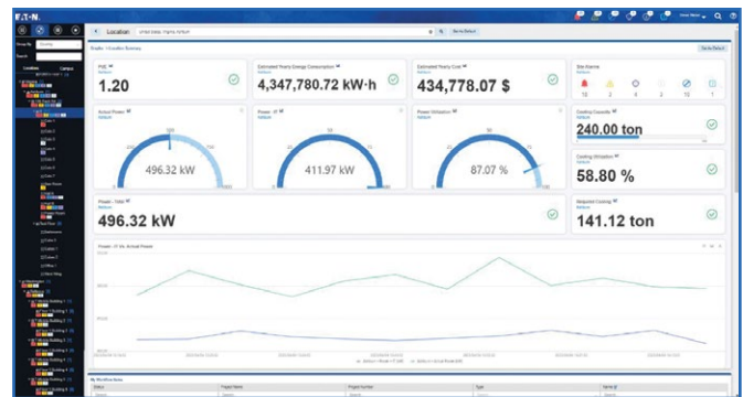
Remote power management dashboard from DITPM software.
