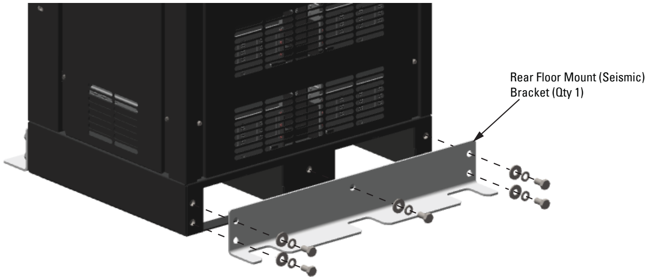
Figure 15. Rear Floor Mount Bracket to Cabinet Installation
