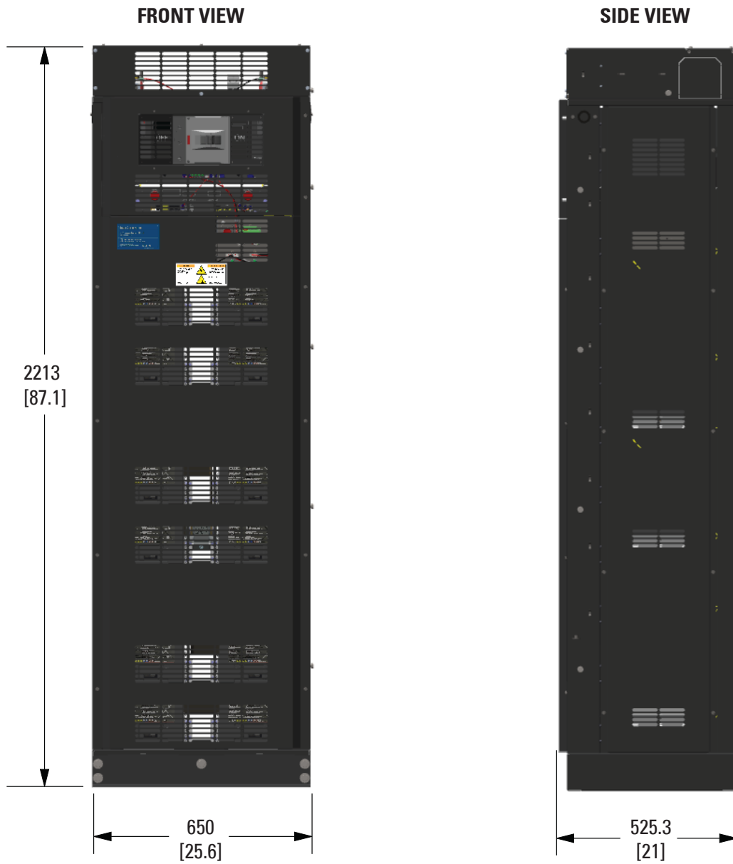
Figure 3. Eaton Samsung Gen 3 Dimensions (Front and Right Side Views)
