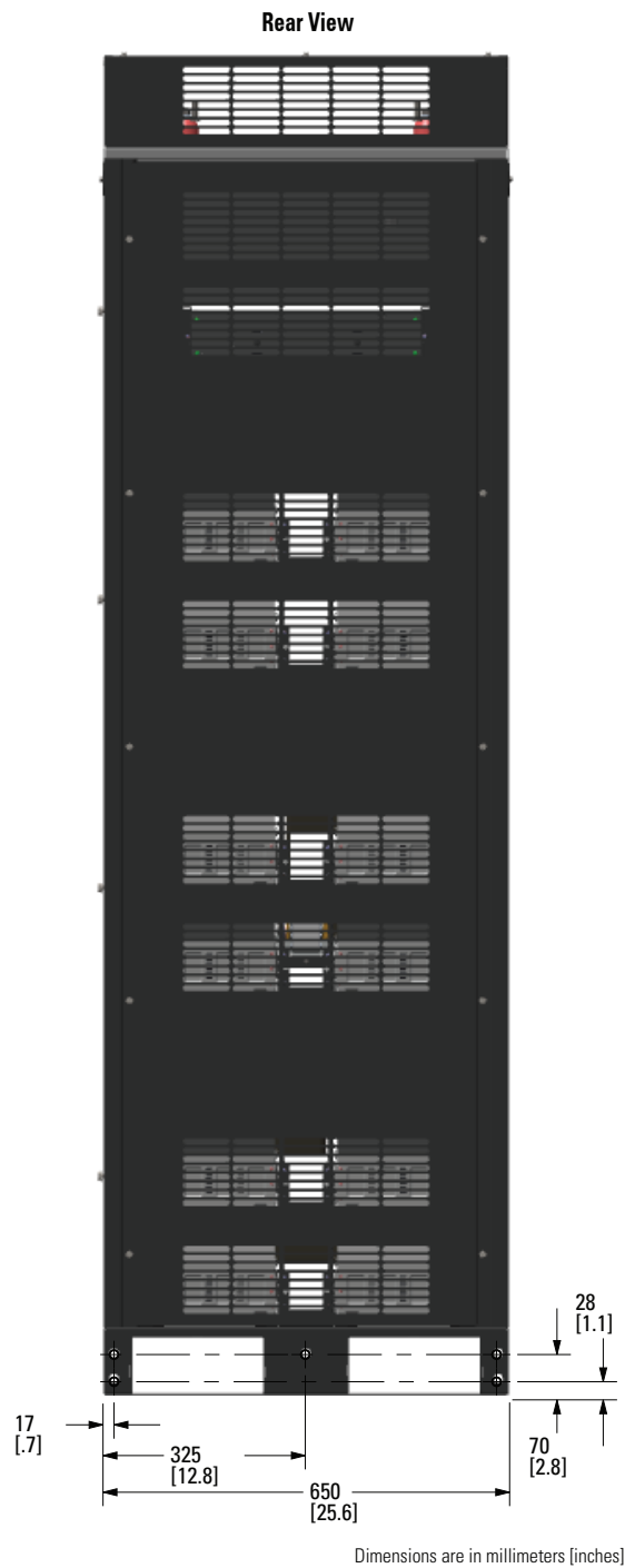
Figure 4. Eaton Samsung Gen 3 Dimensions (Rear View)
