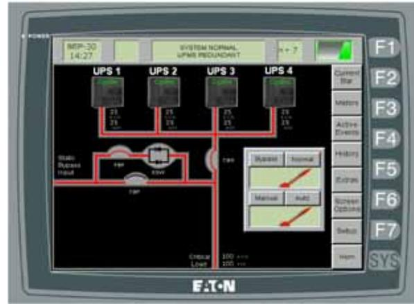
LCD display showing online system with closed system output breaker (CBS), open system bypass breaker (CBP)
