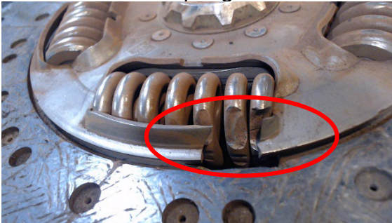
Broken spring cover
