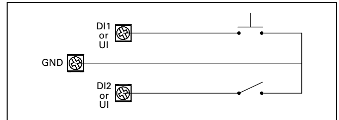
Figure 23.5-4. Maintained or Momentary Dry-Contact Input Connection
