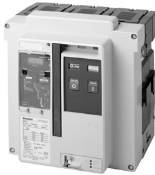
Magnum MDSX current limiting power circuit breakers have fast opening contacts to provide interrupting ratings up to 200 kA at 508 Vac without fuses.
