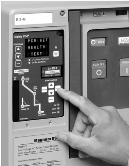
Magnum 1150+ Trip Unit with Arcflash Reduction Maintenance System, 24-Digit LED Display, Programmable Protection, Alarms and Relaying, Power Metering, Power Quality and Alarms, Waveform Capture, Communications and Breaker Health Monitoring
