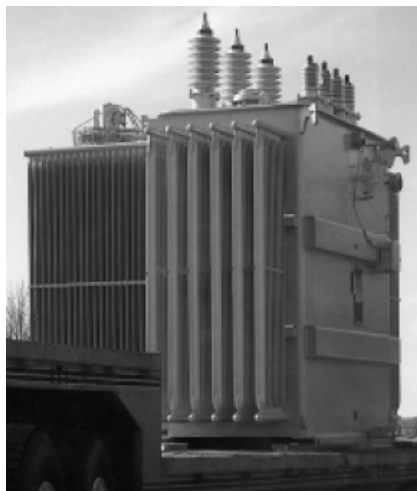
Substation Transformers Feature Cover-Mounted Primary and Secondary Bushings and Can Be Provided with Load (LTC) Changers
