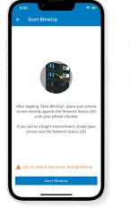
On the EV smart breaker charger, press the "DISPLAY" button and ensure that the Network Status LED is blinking. If it is, then touch the "READY" button on your phone. After reading the instructions on the phone, touch the "START BLINKUP" button.
