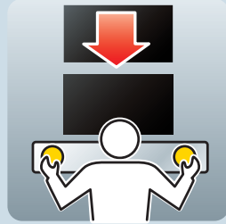
Safe operation with two-hand control
