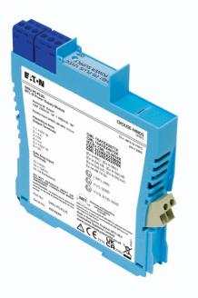
**The MTL 9491-PS-PLUS** takes a 24V DC safe area / Zone 2 supply and produces an intrinsically safe, 12V DC nominal output capable of powering devices mounted in a Zone 0 (ia) or Zone 1 (ib) hazardous area. The 9491-PS-PLUS may be mounted in a safe area or Zone 2 hazardous area.
