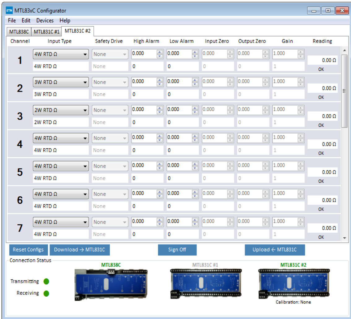
Figure 5: Example MTL831C RTD Configuration
