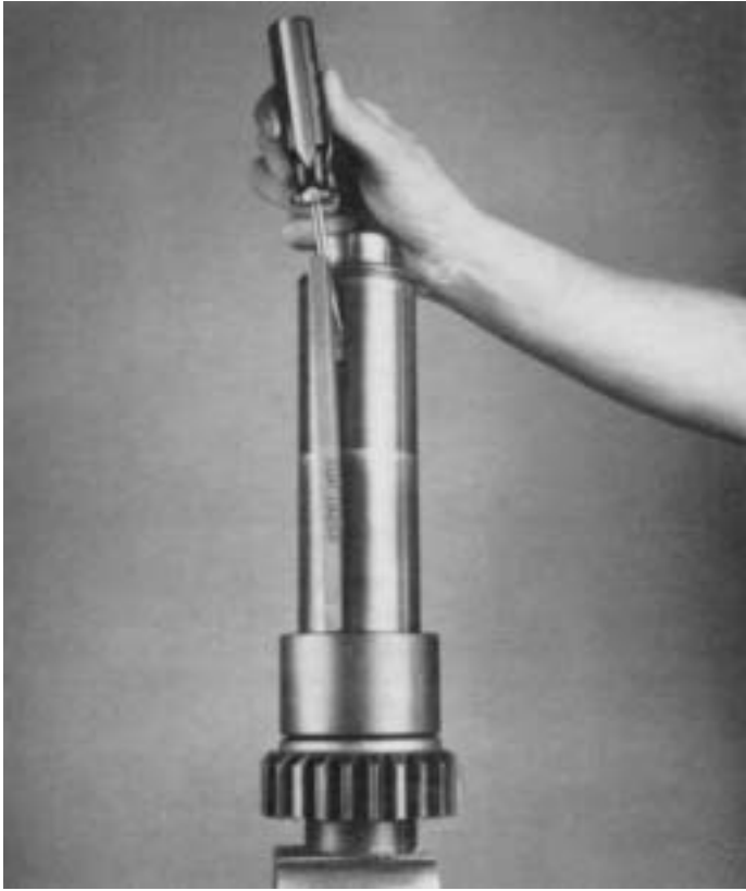
5. If necessary, remove key from countershaft.
