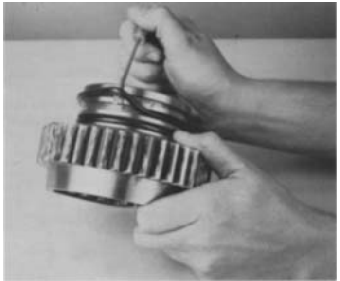
1. If previously removed, install the O-rings on extended front hub of auxiliary drive gear.
