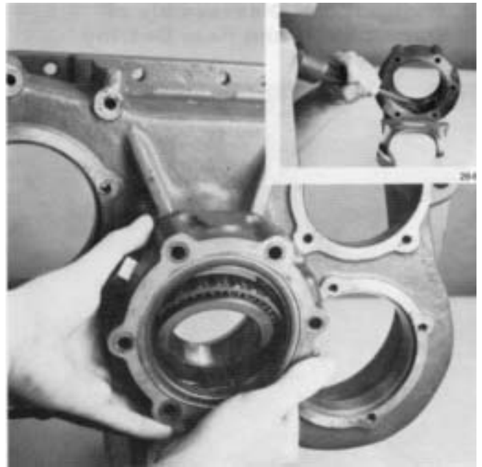
7. Turn out capscrews and remove rear bearing cover. Rear bearing cone will drop from bore in auxiliary plate when cover is removed. If necessary, remove oil seal from cover (inset).
