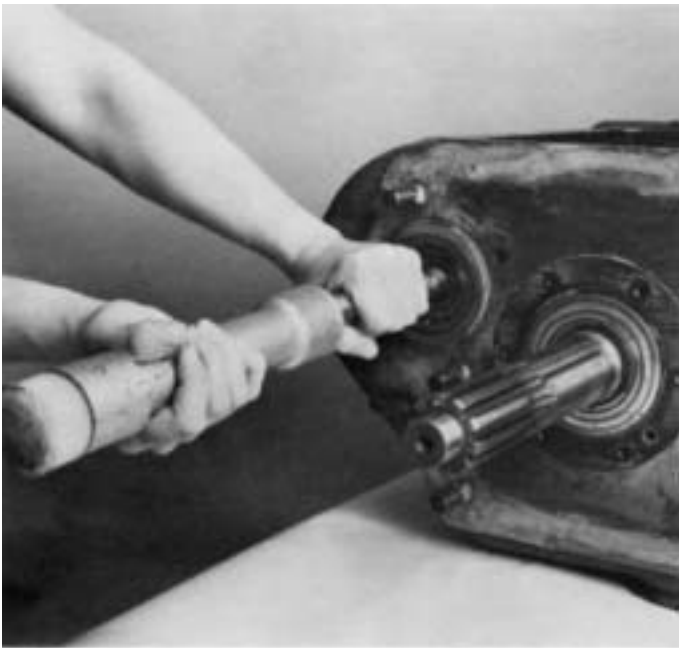
4. Use a soft bar and maul to drive countershaft to the rear as far as possible. This will partially unseat the front bearing. NOTE: The soft bar used should have a flattened end that is large enough so as not to damage holes for roll pin and capscrew.
