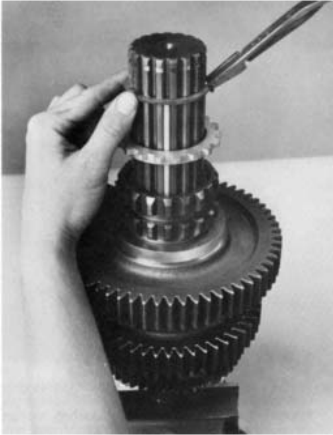
20. Install snap ring in 6th groove of mainshaft to retain key in keyway.
