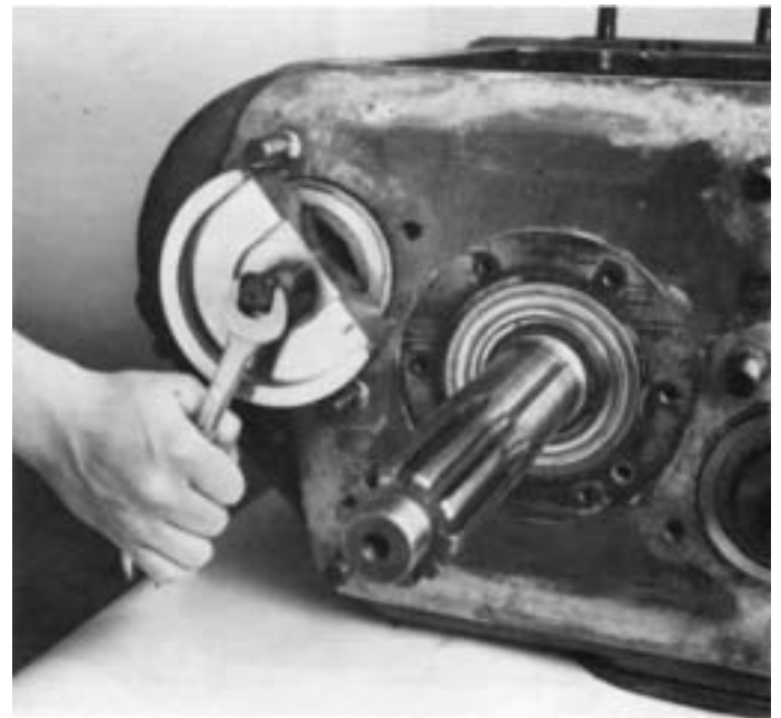
6. Use a bearing puller to remove the countershaft front bearing. NOTE: The bearing inner race of models equipped with roller-type front bearings will remain pressed on countershaft.
