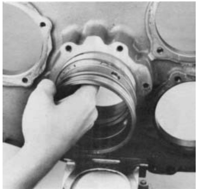
8. Remove two bearing cups and outer spacer from bore in auxiliary plate.
