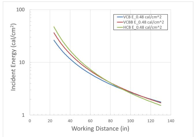
Fig. 6 Incident Energy vs. Working Distance
