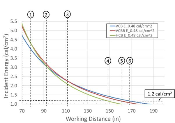
Fig. 7 Incident Energy vs. Working Distance
