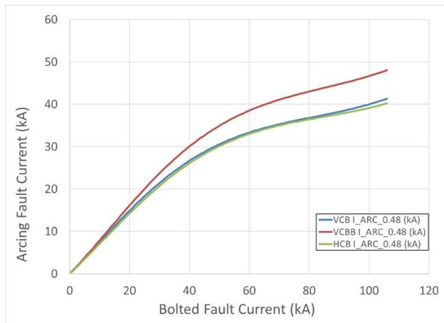
Fig. 1 Arcing Fault Current vs. Bolted Fault Current
