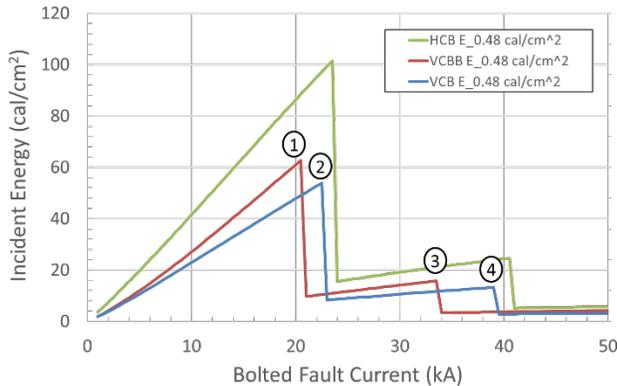
Fig. 3 Incident Energy Plot vs. Bolted Fault Current with Varied Clearing Time
