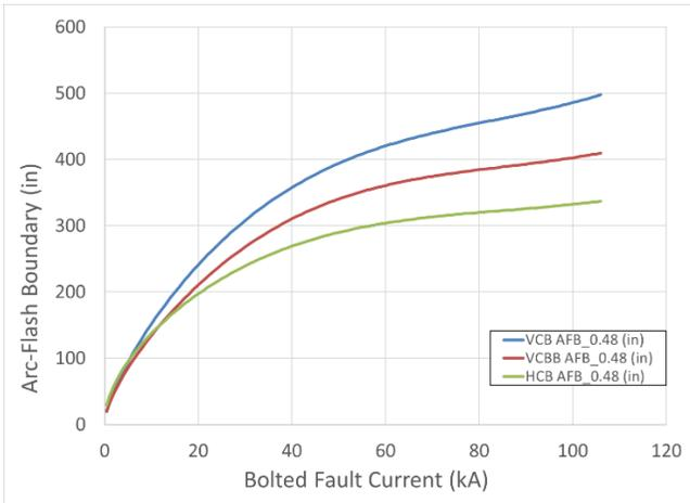
Fig. 4 Arc-Flash Boundary vs. Bolted Fault Current with Fixed Clearing Time
