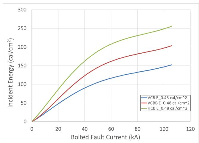
Fig. 2 Incident Energy Plot vs. Bolted Fault Current with Fixed Clearing Time
